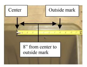
3. The backing plate may be mounted vertically or horizontally depending on which works best for the particular sled. Align the backing plate holes with the outside marks on each side. The top edge of the plate should line up with the top edge of the sled when mounted vertically or 1" down from the sled top edge when mounted horizontally. Drill out the top and the bottom holes using a 5/16 drill bit.
