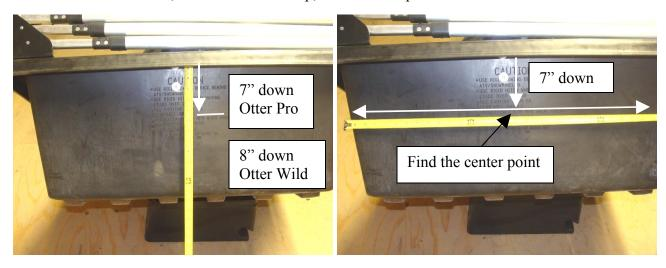
2. From the center point measure 3/4" to the left and place a mark. Drill a hole at that mark using an 11/32" drill bit or just over 5/16". Place the hitch receiver into position and put a 5/16 bolt through the receiver and the hole. Lightly tighten into place. Make sure the receiver is level and then drill out the second hole.
