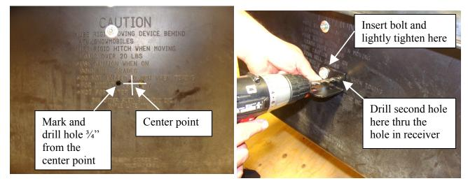
3. Remove the bolt from the receiver and line up the inside backing plate with the holes in the sled and the holes in the receiver. Insert the bolts and washers through the inside plate and the receiver and tighten down using the nylock nuts.
