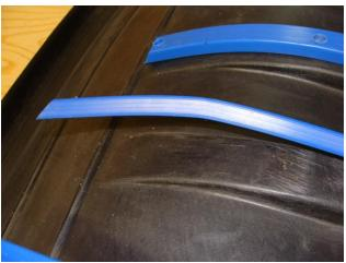
2. Center the strip on the rib, and using the hole in the hyfax strip as a guide, drill a hole into the sled using a 1/8" drill bit. Attach the strip to the sled using the provided allen screw and small washer. Using an allen bit and drill/driver will allow the screw to be driven into the small hole in the plastic. Turn in until just barely tight. This may be done by hand but will require more effort.
